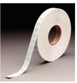
for sterilisation facilities to ensure that products have been exposed to the sterilisation process. Labels turn from blue to pink after exposure to 121°C for 3-10 mins, or 134°C for 0.5—2 mins.
